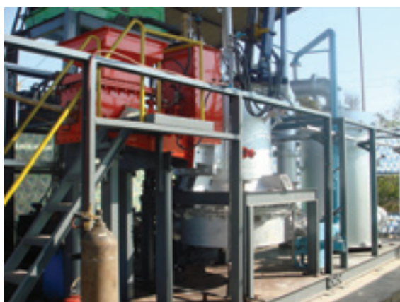
Figure 3: PTDR-100 system commissioned to process a wide range of solid waste streams, including medical waste, industrial process waste (organic and inorganic) and pharmaceutical industry waste
